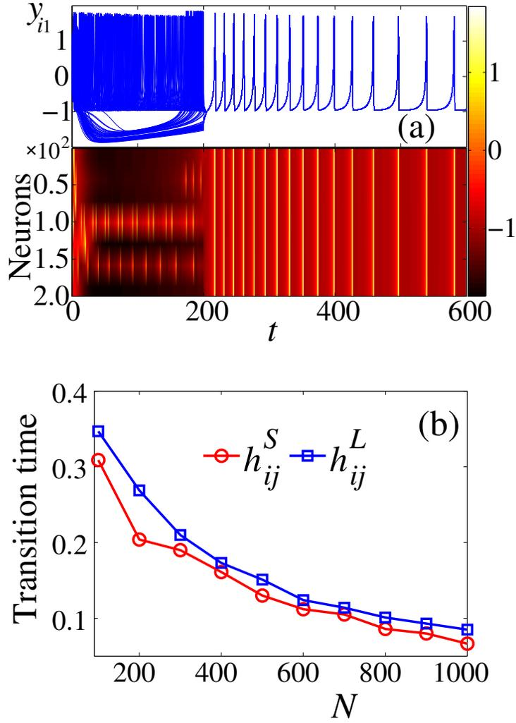
FIG. S4. **Controlled generation synchronization of spiking HR neuronal networks.** (a) Time course (upper) and color map (lower) of all potentials  $y_{i1}$  of a HR neuronal network, where  $\alpha = 1/2$ ,  $k = 0.15$ ,  $h_{ij}^S$  is activated at  $t = 200$ , and the rewiring probability 0.1 and  $N = 200$  are used for generating the small-world network. (b) Synchronization transition time for different values of  $N$ .
