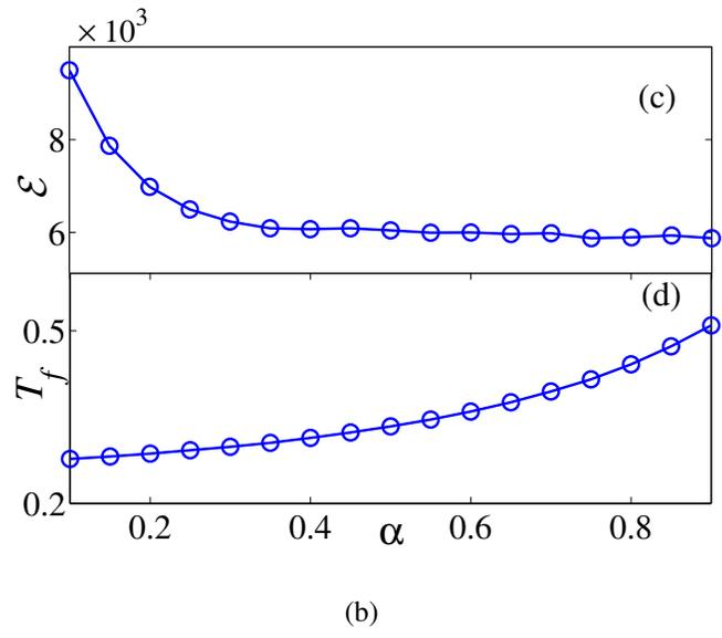
FIG. S1. **Trade-off between required control time and energy cost.** Effects of increasing  $k$  and  $\alpha$  on control time and energy cost for the Florida food-web network: (a) energy cost versus  $k$ , (b) control time versus  $k$ , (c) energy cost versus  $\alpha$ , and (d) control time versus  $\alpha$ . The initial state values are randomly taken from the interval  $[0, 5]$ .
