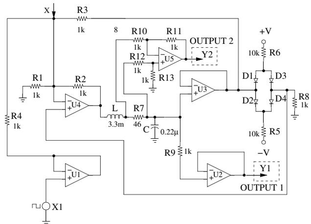
FIG. 2. Young-Silva circuit implementation of the Duffing oscillator. A differential amplifier (U5) was added to generate a single output proportional to the voltage across (R7) in order to visualize the phase plot of the voltage at Y1 versus that at Y2 on an oscilloscope.
