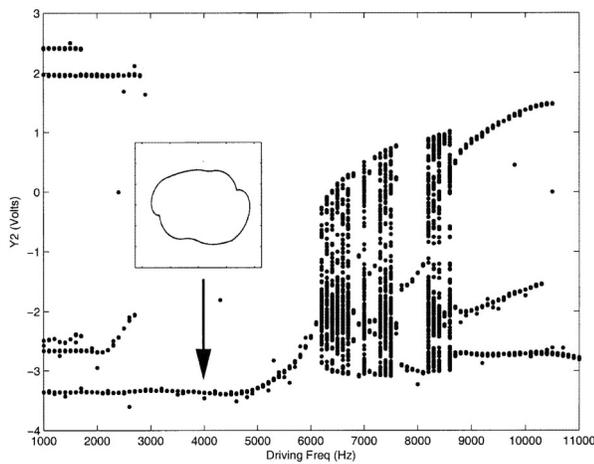
FIG. 3. Experimental bifurcation diagram for the Duffing circuit. The vertical arrow indicates the initial period-1 state of the system that is to be brought into chaos using a resonant perturbation.
