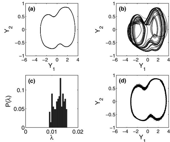
FIG. 4. (a) Phase-space plot of a periodic attractor from the Duffing circuit, (b) induced chaotic attractor under resonant driving, (c) histogram of the largest Lyapunov exponent from the induced chaotic attractor, and (d) attractor due to noisy driving, which is nonchaotic. The units of  $Y_1$  and  $Y_2$  in (a), (b), and (d) are in volts.
