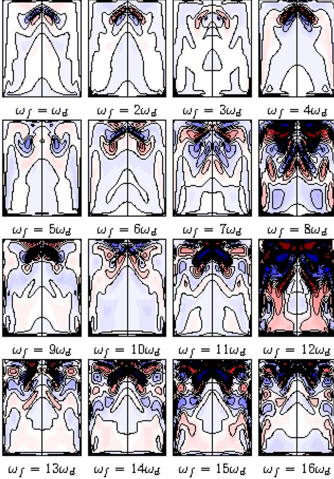
FIG. 5. (Color online) Vorticity field under decelerated parameter ramping. For  $P = 1/2$ , snapshots of the azimuthal vorticity field for various values of  $\omega_f$  at different instants in time, where  $\omega_d = 2\omega_b/3$ . Relatively strong vorticity fields are observed for  $\omega_f(t) = 8\omega_b$ ,  $12\omega_b$ , or  $15\omega_b$ , as in the corresponding stationary system (cf. Fig. 1).
