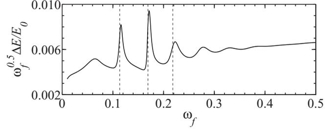
FIG. 2. Multiple resonances in the stationary driven flow system. Normalized peak-to-peak amplitude of the kinetic energy versus the forcing frequency  $\omega_f$  for  $A = 0.01$  in the stationary driven system, where each dashed line indicates a Hopf frequency  $\omega_i$  ( $i = 1, 2, 3$ ).
