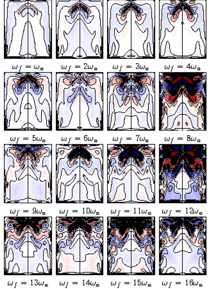
FIG. 6. (Color online) Vorticity field under accelerated parameter ramping. For  $P = 2$ , snapshots of the azimuthal vorticity field for various values of  $\omega_f$  at different instants in time, where  $\omega_a = \omega_b/3$ . Relatively strong vorticity fields are observed for  $\omega_f(t) = 8\omega_b$ ,  $12\omega_b$ , or  $15\omega_b$ , as in the corresponding stationary system (cf. Fig. 1).
