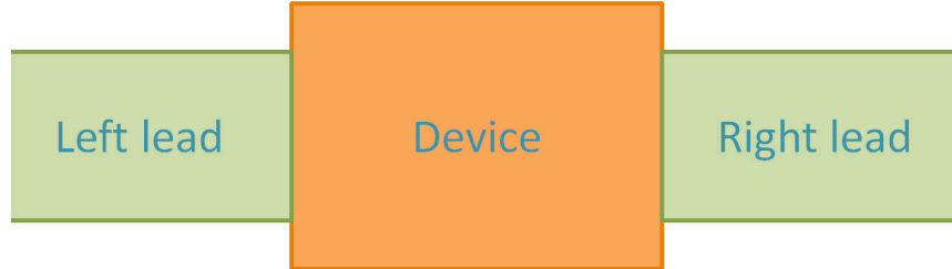
Fig. 3 A conceptual visualization of the separation of the entire system into a pair of leads plus the actual device.
