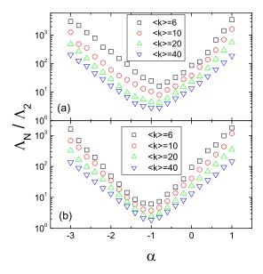
FIG. 7. (Color online) For (a) symmetric coupling scheme and (b) asymmetric coupling scheme, ratio of the largest eigenvalue and the second lowest eigenvalue of the coupling matrix as a function of  $\alpha$  for different average degree  $\langle k \rangle$  of scale-free networks of N=2000 nodes. Each data point is the results of averaging over 20 random network realizations.
