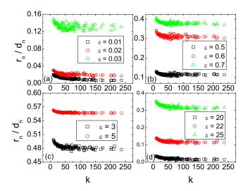
FIG. 2. (Color online) Nodal order parameter  $r_n/d_n$  as a function of node degree k for (a)  $\alpha$ =0, (b)  $\alpha$ =-0.4, (c)  $\alpha$ =-0.6, and (d)  $\alpha$ =-1.0 for different values of  $\varepsilon$  close to the onset of partial synchronization. The network size is 2000 and the average degree is  $\langle k \rangle$ =20.
