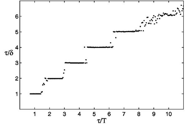
FIG. 3. Dependence of the average interval  $\delta$  between large pulses on the ratio  $\tau/T$ . A pulse is considered “large” when its peak is above the energy surface of the ECM's, as given by Eq (2):  $E_i^2 > (P - N_i)/(2N_i + 1)$ . The system parameters are  $\alpha = 6$ ,  $\tau = 700$ ,  $\eta = 0.07$ ,  $\phi_0 = 0$ , and  $P = -0.012$ . Each dot represents a median value of 3000 time intervals.
