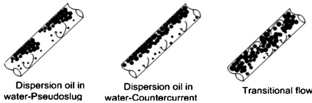
FIG. 5. Experimentally observed flow patterns: from left to right are PS, CT, and TF, respectively.
