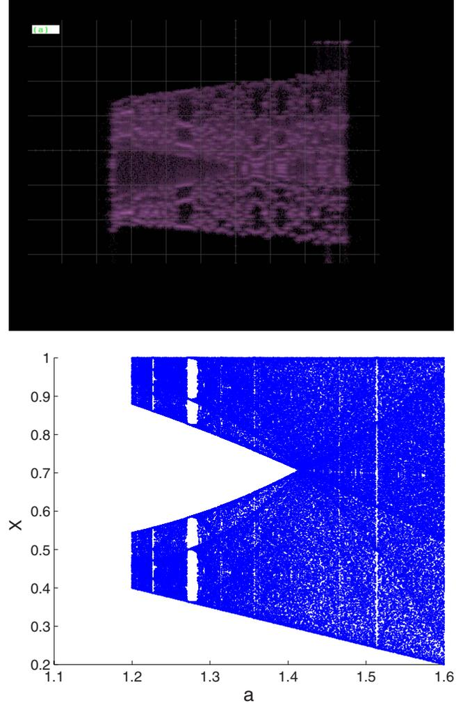
FIG. 8. (Color online) (a) Experimentally obtained bifurcation diagram of the circuit. The full screen sweep is 100 ms, which corresponds to sweeping through the parameter  $a$  in Eq. (14) in the range [1.2,1.6]. (b) Numerically computed bifurcation diagram of the smoothed tent map for  $\beta=100$ .
