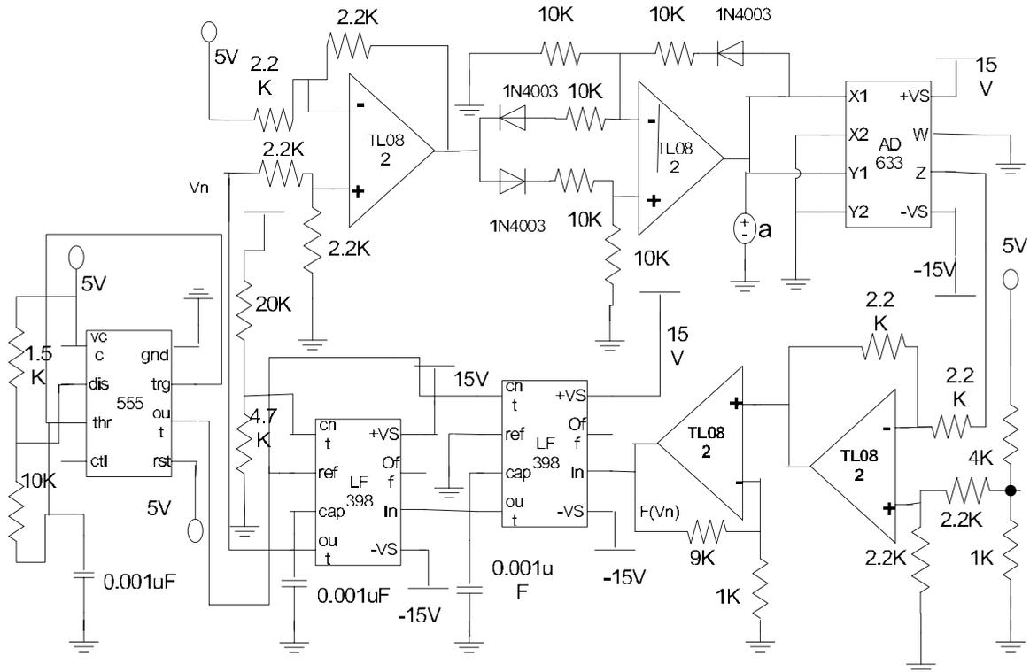
FIG. 7. Schematic of the circuit realization of Eq. (14). The voltage  $V_n$  corresponding to the dynamical variable  $x$  is indicated.
