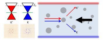
FIG. 2. A schematic illustration of geometric valley Hall effect (gVHE) induced by skew scattering from impurities (gray shaded disks). This type of Hall effect is *mixed* that is mediated by the inherent singular Berry flux and manifests itself with exceptional valley skew scattering from valley-independent scalar-type impurities.
