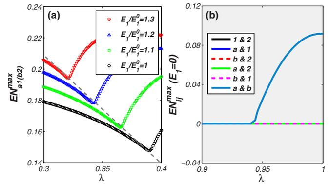
FIG. 5. (Color online) Effect of driving laser power on the transition point: (a) Maximum LN values between the mechanical modes for laser amplitude  $E_1 = E_1^0, 1.1E_1^0, 1.2E_1^0, 1.3E_1^0$  (from lower to upper curves), where  $E_1^0/\omega_m = 1.351 \times 10^4$ . The gray dashed line indicates a linear relation between the critical points  $\lambda_c$  and  $E_1$ . (b) Maximum LN values between the optical modes in the two cavities versus  $\lambda$  for  $E_1 = 0$ .
