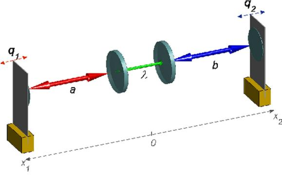
FIG. 1. (Color online) Schematic illustration of our system of two coupled optomechanical cavities. The coupling between the two subsystems is realized by an optical fiber with  $\lambda$  being the coupling parameter. The displacements of the cantilevers are denoted by  $q_{1,2}$ .
