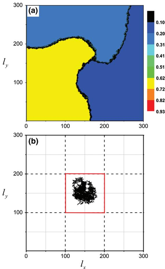
**Fig. 1** (Color online) For  $\varepsilon = 0.166$ , the three-armed spiral wave pattern generated in the regular lattice of  $300 \times 300$  coupled chaotic maps. **a** A snapshot of the system dynamics taken at the iteration step  $n = 2.5 \times 10^3$ . **b** The random motion of the spiral tip inside the central area marked by the (red) square
