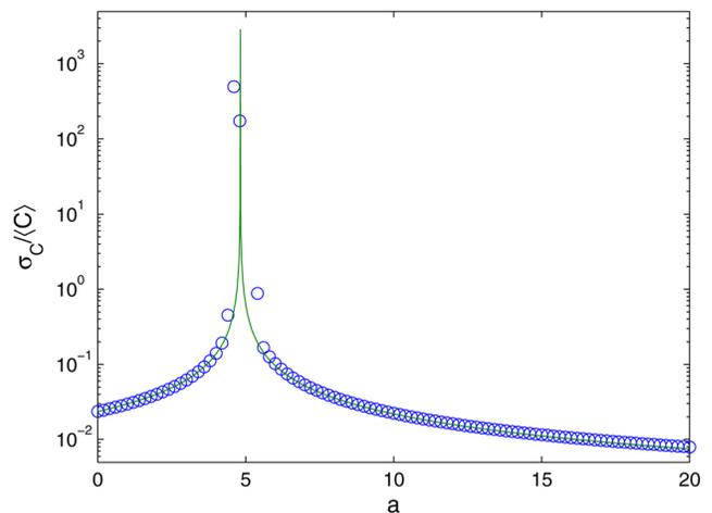
FIG. 3. (Color online) For an ensemble of  $10^6$ ,  $100 \times 100$  random matrices, ratio  $R_C \equiv \sigma_C / \langle C \rangle$  versus  $a$ . Open circles are results from direct computation, and the solid curve is from theoretical prediction Eq. (8).
