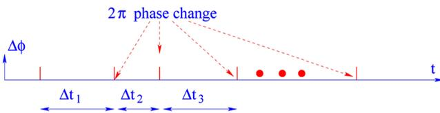
FIG. 1. (Color online) Schematic illustration of the definition of APST, where  $\Delta\phi(t)$  is the phase difference between signals from an arbitrary pair of channels. Each  $\Delta t_n$  ( $n=1, \dots$ ) represents a time interval, where  $\Delta\phi$  remains bounded within  $2\pi$ . The APST is  $\tau \equiv \lim_{n \rightarrow \infty} (1/n) \sum_{i=1}^n \Delta t_i$ .
