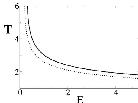
FIG. 3. Average delay time versus the energy. The time diverges as the particle energy approaches the threshold value  $E_e$  from above. The dotted curve is for the nondissipative case. The solid curve is for dissipative case with  $\alpha = \beta = 10^{-3}$ .
