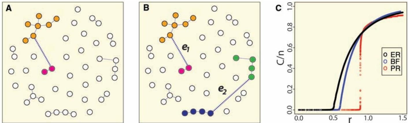
16). In contrast, the rule selecting the edge minimizing the sum of the component sizes instead of the product would select  $e_2$  rather than  $e_1$ . (C) Typical evolution of  $C/n$  for ER, BF (a bounded size rule with  $K = 1$ ), and PR, shown for  $n = 512,000$ .
